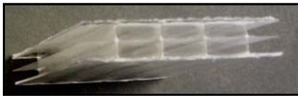
A sample of triple-thick polycarbonate glazing.
